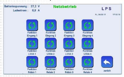
On the system you can connect 8 light switches. 4 inputs are for potential free contacts (Input 1-4), the other 4 inputs (LSAA1-LSAA4) must be connected to the terminals in the system with 230V 50H. (see terminal plan). So that the light switches can be used and certain circuits, groups of luminaire or even individual luminaire can be switched on or off, they must be programmed.
